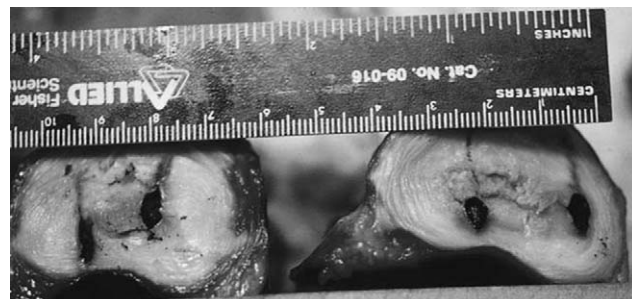
Fig. 4. Laser tracts formed in nucleus pulposus by 1000 J of laser energy at a 1320 nm on the left, and a 1060 nm Nd:YAG laser on the right.
